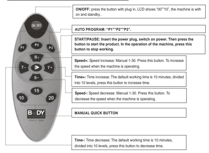
NOTE: The effective reception range of the remote control signal is 2.5 meters, the infrared emission indicator of the controller should be aligned the infrared receiving window on the product.
