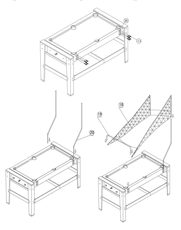
7. Assemble the net slide. Carefully lay out the main parts, taking time to ensure they are the right way round, and assemble using the parts shown. Fit all the fixings first, only loosely and once all are fitted, go back and tighten them all securely.
