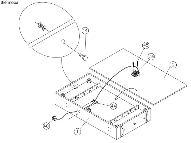
2. Turn the playing surface over and fix in place using 4x #12 screws. Fit the goal brackets to the ends of the table as shown.
