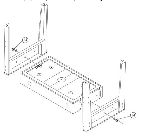
5. Assemble the leg braces. Carefully lay out the main parts, taking time to ensure they are the right way round, and assemble using the parts shown. Fit all the fixings first, only loosely and once all are fitted, go back and tighten them all securely.
