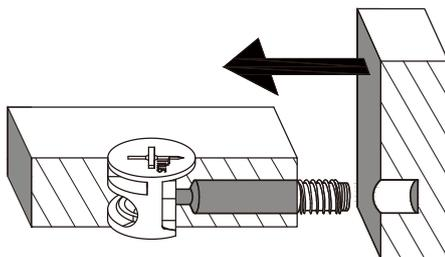
TURN THE CAM IN A CLOCKWISE DIRECTION
