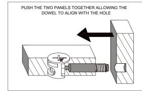
TURN THE CAM IN A CLOCKWISE DIRECTION
