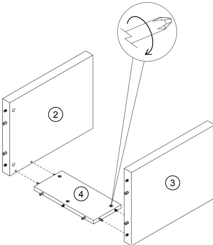
PUSH THE TWO PANELS TOGETHER ALLOWING THE DOWEL TO ALIGN WITH THE HOLE
