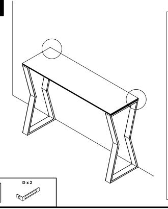
Move the console into its location of intended use next to a wall. The wall bracket (D) may also require some adjustment to fit correctly depending on any obstructions behind the console such as skirting boards, picture rails etc.
