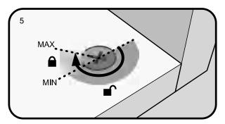
The panels are locked when each cam is turned to between 1/2 and 2/3 of a full turn (Maximum rotation)
