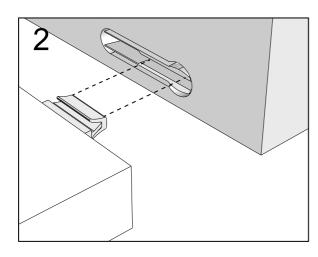
Push connector into housing to be jointed.
