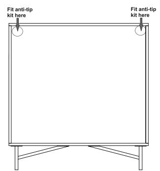
Note: Fit the anti-tip straps on both top corners of the rear side of the product and fix the other end of the strap to wall
