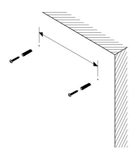
Insert an appropriate wall plug into each hole. Insert the screws and tighten, leaving the screw head axposed by 1/4 inch (6mm)
