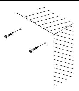
Insert an appropriate wall plug into each hole. Insert the screws and tighten, leaving the screw head exposed by 1/4 inch(6mm)
