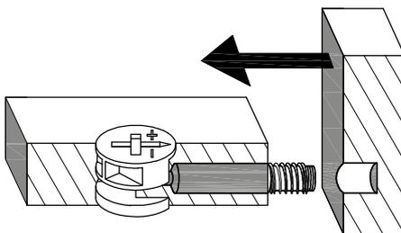
TURN THE CAM IN A CLOCKWISE DIRECTION
