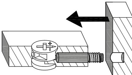
TURN THE CAM IN A CLOCKWISE DIRECTION
