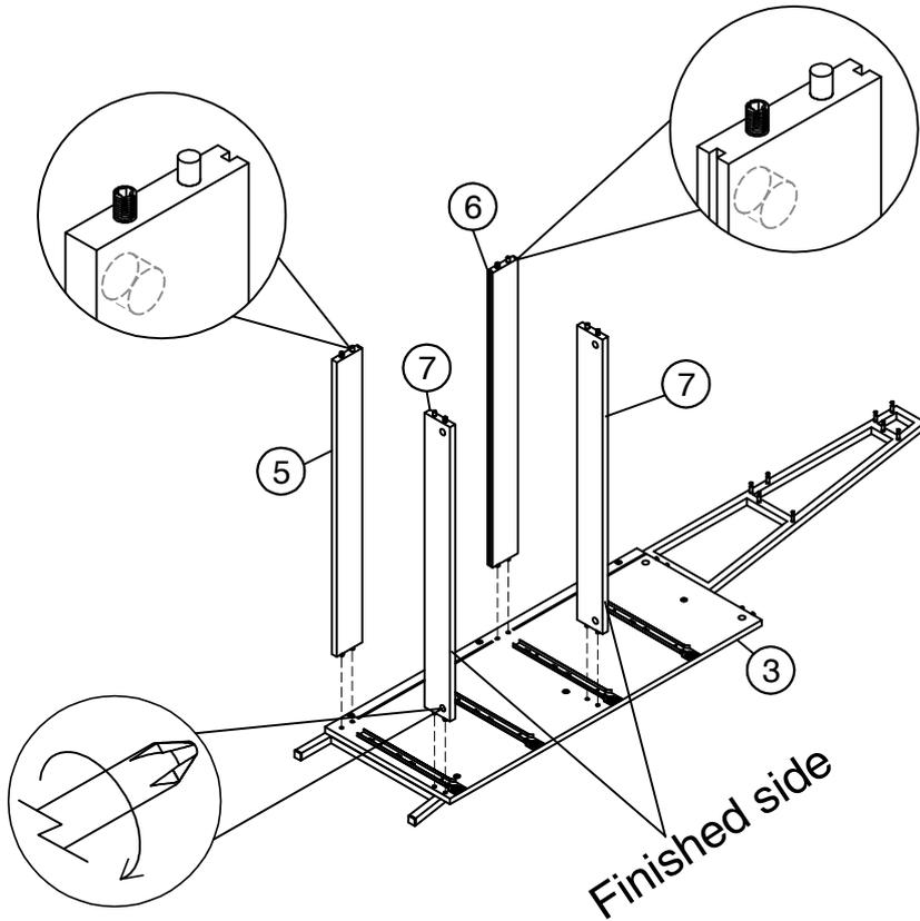
PUSH THE TWO PANELS TOGETHER ALLOWING THE DOWEL TO ALIGN WITH THE HOLE
