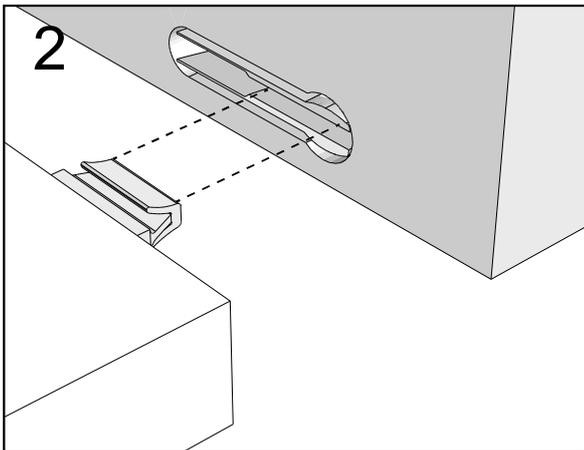
Push connector into housing to join.
