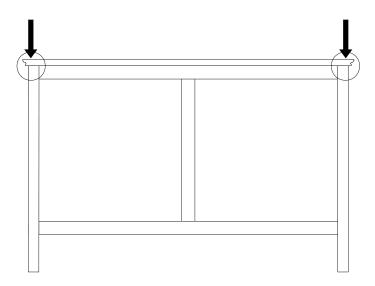
Note: Fit the anti tip straps on both top corners of the rear side of the product and fix the other end of the strap to wall.
