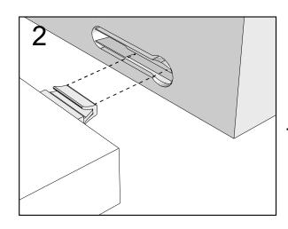
Push connector into housing to join.
