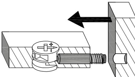
TURN THE CAM IN A CLOCKWISE DIRECTION
