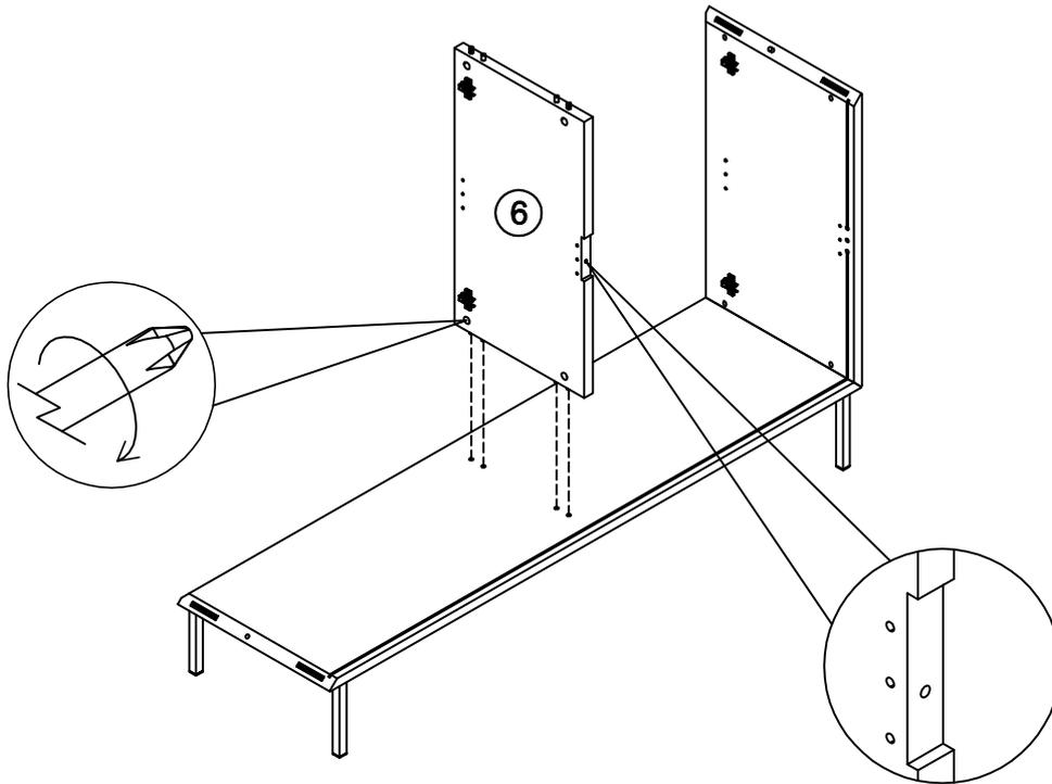
PUSH THE TWO PANELS TOGETHER ALLOWING THE DOWEL TO ALIGN WITH THE HOLE
