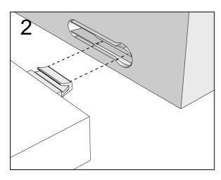
Push connector into housing to be jointed.
