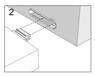
Push connector into housing to be jointed.
