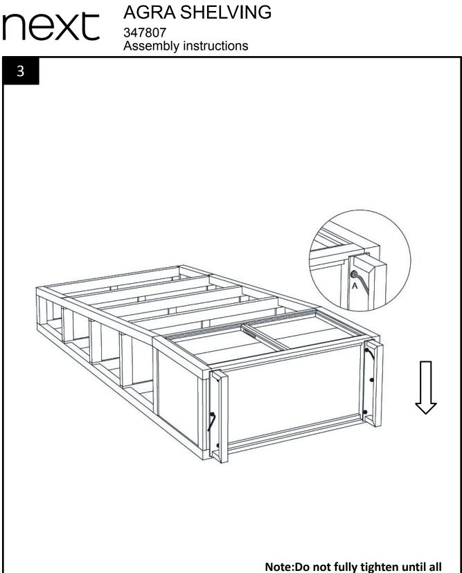
Note:Do not fully tighten until all fittings are in position.
