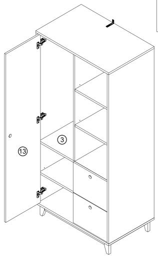
Note: Lock the hinge after adjustment! If need be, add screws on the mounting plate to strengthen it.
