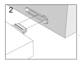
Push connector into housing to join.
