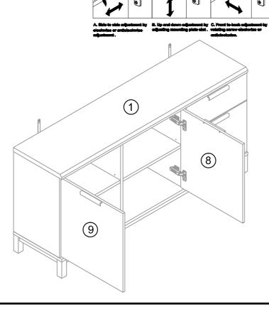
Lock the hinge after adjustment if need be, add screws on the mounting plate to strengthen it.
