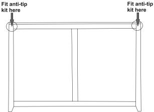
Note: Fit the anti-tip straps on both top corners of the rear side of the product and fix the other end of the strap to wall
