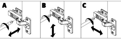
A. Side to side adjustment by clockwise or anticlockwise adjustment. B. Up and down adjustment by adjusting mounting plate slot .
