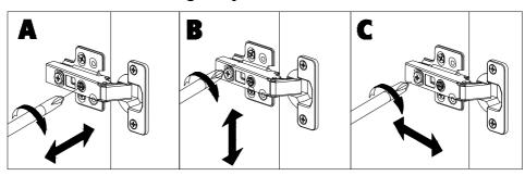
A. Side to side adjustment by clockwise or anticlockwise adjustment.
