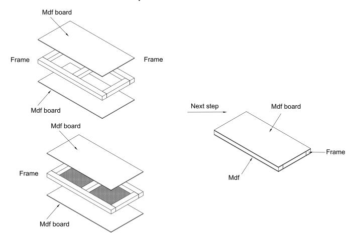
The centre of Hollow board & Honeycomb board is hollow. To avoid damaging the hollow board/honeycomb board, we suggest you not step on the hollow board/honeycomb board or not put other part on the board on the end when you assemble the product.
