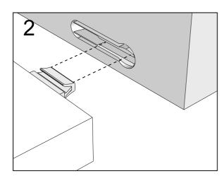
Push connector into housing to be jointed.
