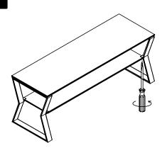
Adjust the plastic screw of the shelf clips (D) with a screwdriver as shown.
