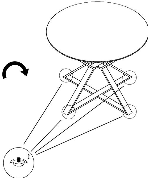
If table is not level, adjust it with the adjustable feet.
