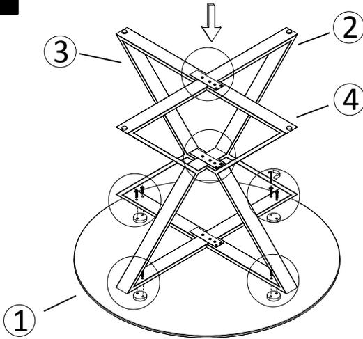
With 2 people carefully align the legs as shown. Finger tighten the bolts (B) ensuring no gaps between legs 2, 3 and 4. Using the allen key C, first fully tighten bolts A and then proceed to fully tighten bolts B.
