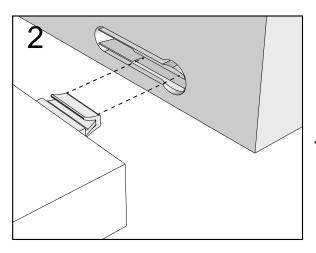
Push connector into housing to join.
