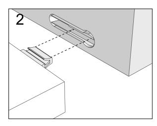
Push connector into housing to be jointed.
