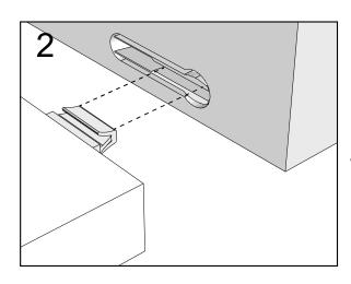
Push connector into housing to join.
