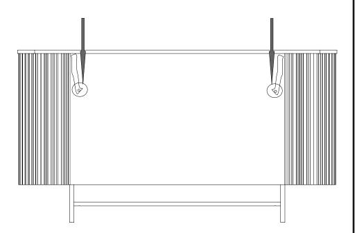
Note: Fit the other end of anti-tip straps provided on both top corners of the rear side of the product to wall
