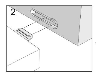
Push connector into housing to join.
