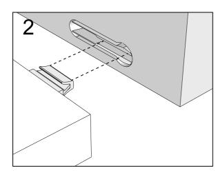
Push connector into housing to be jointed.
