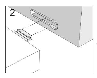
Push connector into housing to join.
