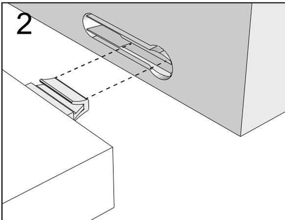
Push connector into housing to join.
