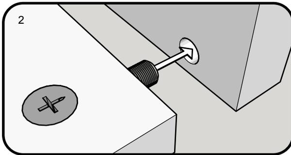
Push the pins into the holes in the panel to be joined.
