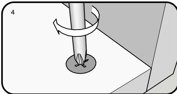
Use a cross-point screwdriver (PH2 or PZ2 is ideal) to tighten the cams and lock the panels together.
