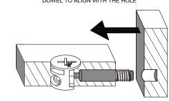
TURN THE CAM IN A CLOCKWISE DIRECTION
