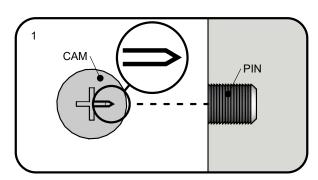
Line up the arrow on the CAM with the PIN.
