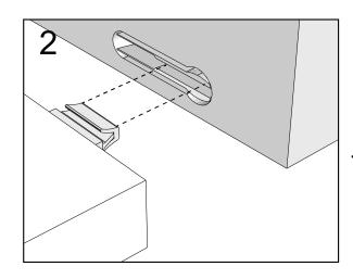
Push connector into housing to join.
