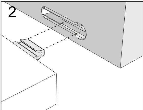
Push connector into housing to join.
