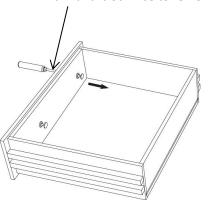
Note:Open the drawer to its maximum and remove the knob from back of the drawer front and fit to front.
