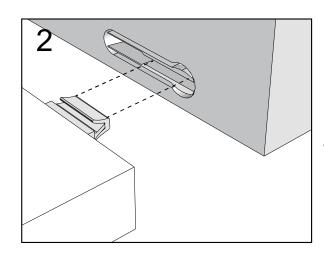
Push connector into housing to join.
