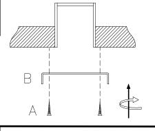
Attach mounting strap to the ceiling using screws supplied. The screws should penetrate a ceiling joist by at least 25 mm.
