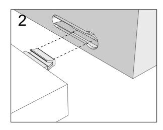
Push connector into housing to be jointed.
