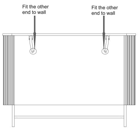
Note: Fit the other end of anti-tip straps provided on both top corners of the rear side of the product to wall
