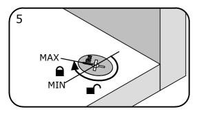
The panels are locked when each cam is turned to between 1/2 and 2/3 of a full turn (Maximum rotation)
