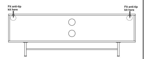
Note: Fit the anti-tip straps on both top corners of the rear side of the product and fix the other end of the strap to wall
