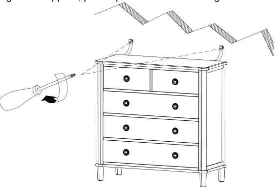
Always ensure that the wall attachment strap is correctly fitted.
